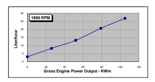
CONVERSIONS: (kWm = BHP x 0.746) (BHP = Engine kWm x 1.34)
